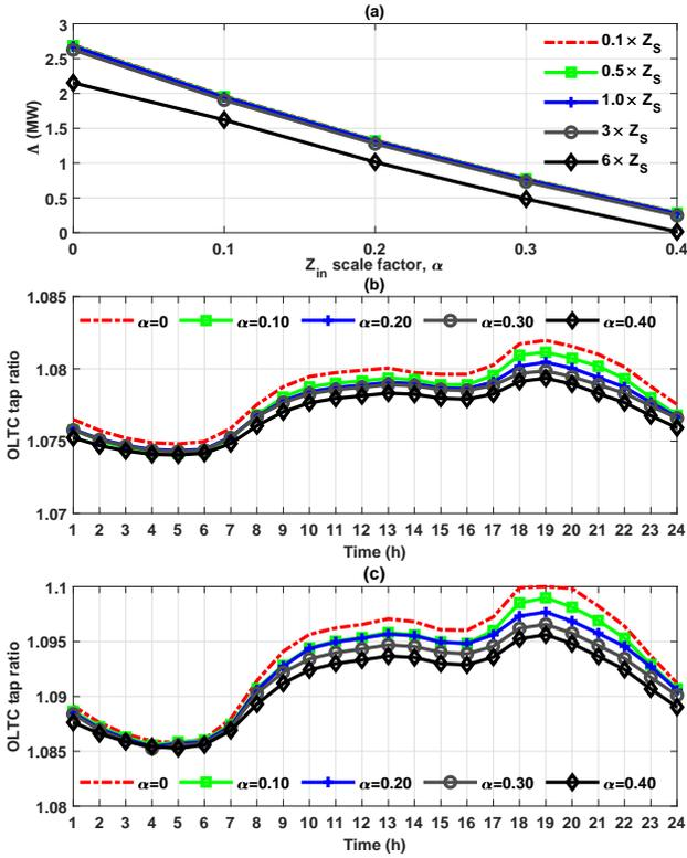
Fig. 13. Impact of  $Z_S$  on minimum HC: (a) HC versus  $\alpha$  for various scales of  $Z_S$ , (b) OLTC's hourly tap settings for  $0.1 \times Z_S$ , (c) OLTC's hourly tap settings for  $6 \times Z_S$ ,
