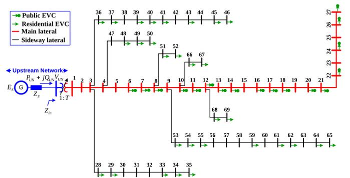
Fig. 3. Single-line diagram of the IEEE 69-bus feeder.
