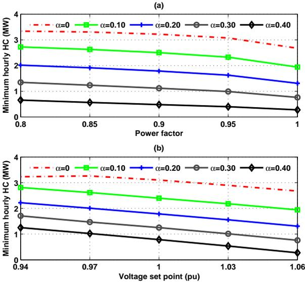
Fig. 11. Sensitivity of HC, ( $\Delta$ ) in different levels of  $\alpha$ , (a) Vs DERs power factor, (b) Vs, OLTC's voltage set point
