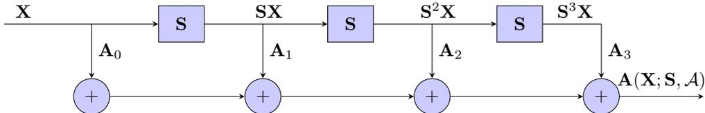
Figure 1. The graph filter performs successive local node exchanges with neighbors, where the  $k$ -shifted signal  $\mathbf{S}^k \mathbf{X}$  collects the information from  $k$ -hop neighborhood (shown by the increasing disks), and aggregates these shifted signals  $\mathbf{X}, \dots, \mathbf{S}^K \mathbf{X}$  with a set of parameters  $[b_0^{11}, \dots, b_K^{11}]^\top$  to generate the higher-level feature that accounts for the graph structure up to a neighborhood of radius  $K$ .
