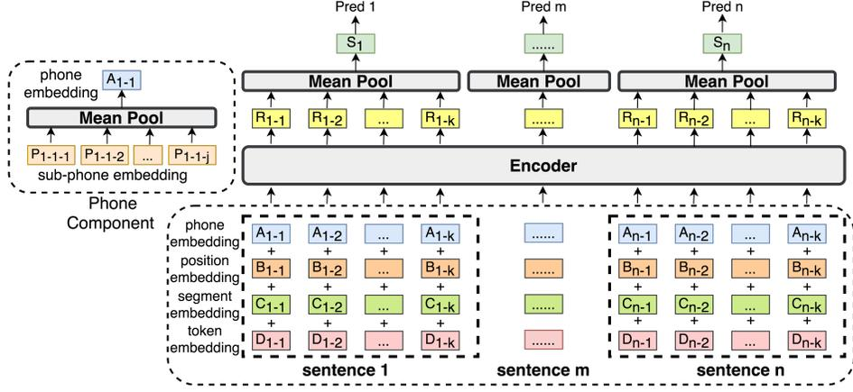
(a) A diagram illustrating our proposed **SeqModel** for document segmentation. The phone component on the left provides an enlarged view for illustrating how phone embeddings are computed to improve the robustness of the proposed model for segmenting spoken documents (Section 2.3).
