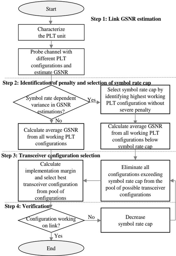
Fig. 1: Extended channel probing flowchart
