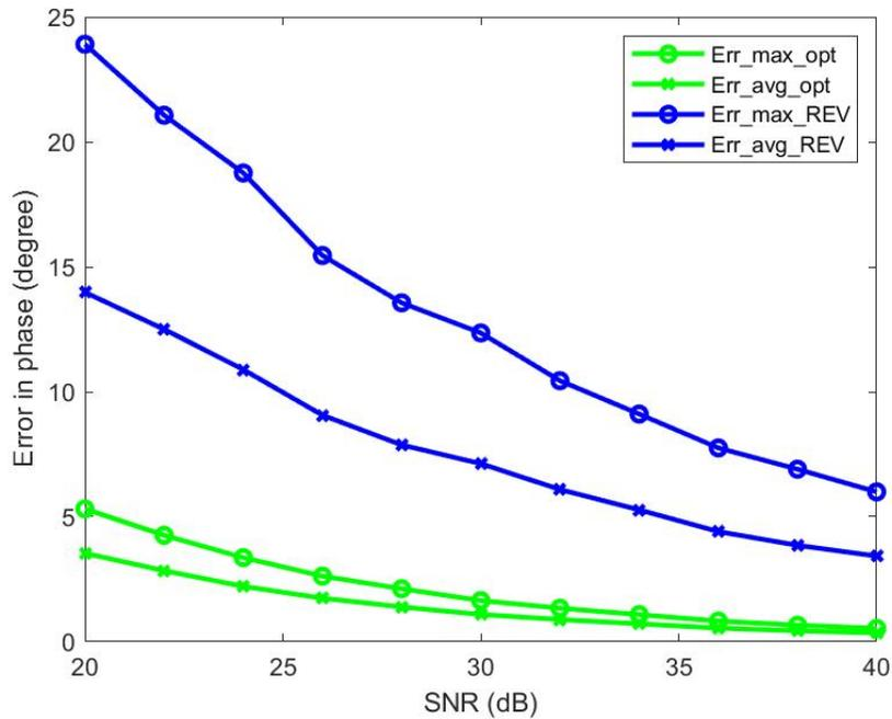
Fig. 12. Comparison with REV method for error in phase calibration
