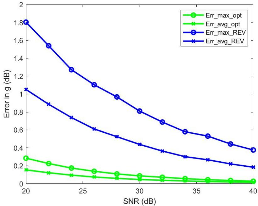
Fig. 13. Comparison with REV method for percentage error in gain calibration.
