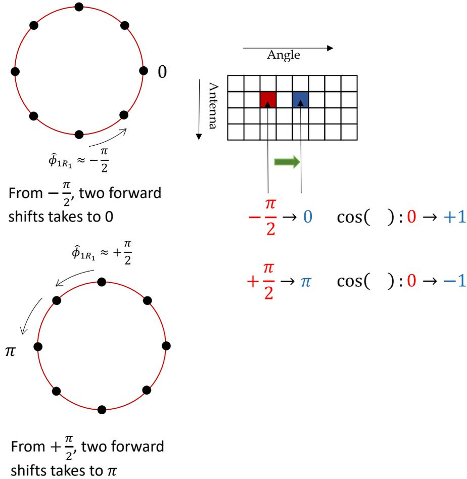
Fig. 6. Resolving the sign of  $\hat{\phi}_{1R_1}$  by looking at the value of  $\cos(\hat{\phi}_{1(R_1+2)\bmod 8})$
