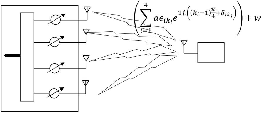
Fig. 1. Illustration of measurement with all antennas turned ON
