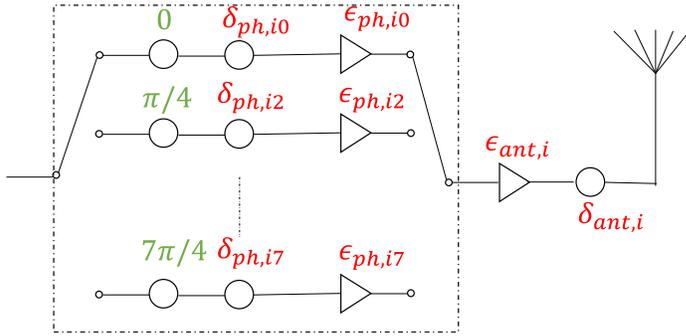
Fig. 2. Illustration of errors for  $i^{\text{th}}$  antenna.
