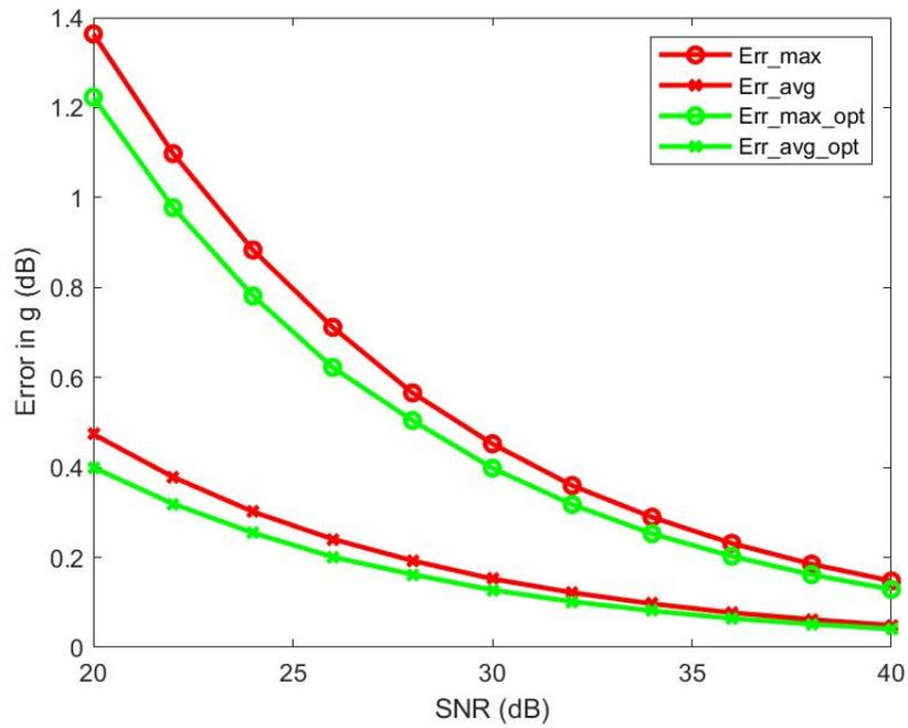
Fig. 11. Comparison of percentage error in gain calibration.
