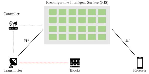
Figure 1. Considered RIS-based wireless communication system consisting of a  $M$ -antenna BS simultaneously serving in the downlink  $K$  single-antenna mobile users.
