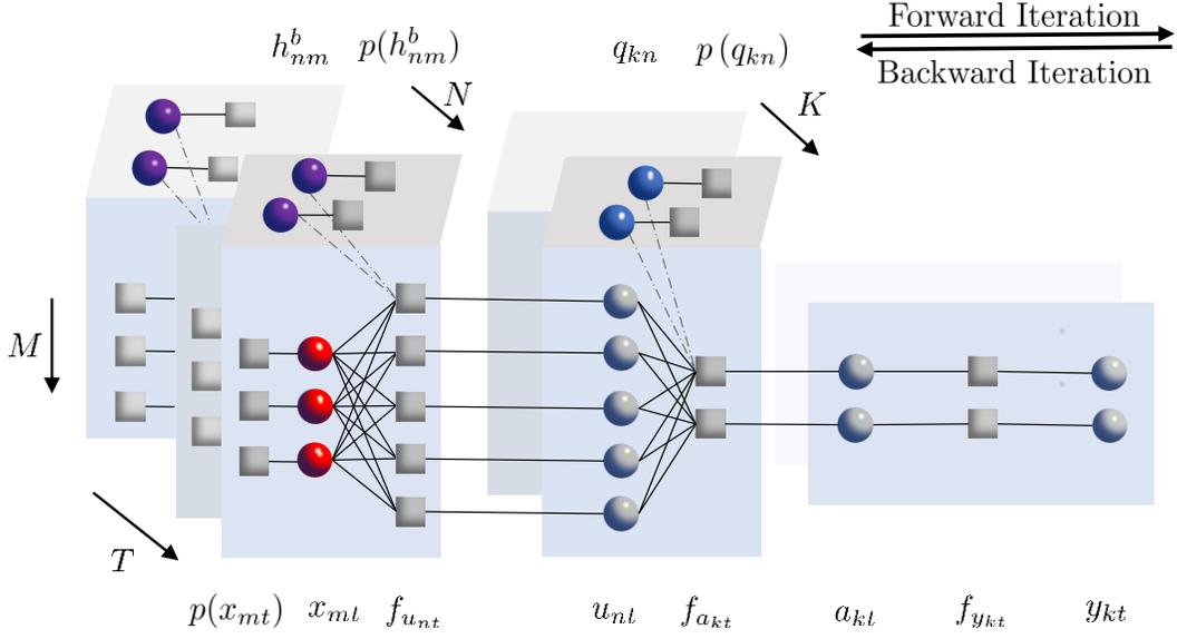
Figure 2. The factor graph of the joint channel estimation and signal recovery in RIS-assisted wireless communication systems.
