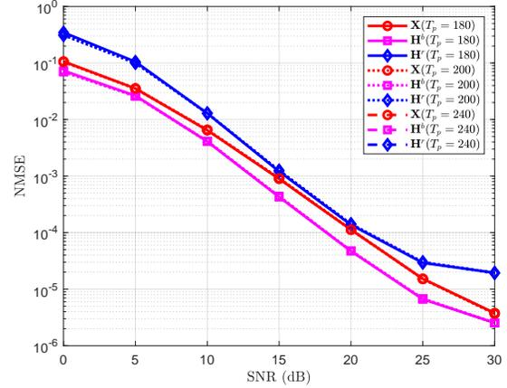
Figure 4. NMSE performance comparisons of the BAMP two-layer algorithm versus the SNR in dB for  $M = 100$ ,  $K = 500$ ,  $N = 100$ ,  $T = 600$  and various values of  $T_p$ .
