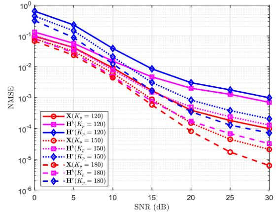
Figure 5. NMSE performance comparisons of the BAMP two-layer algorithm versus the SNR in dB for  $M = 100$ ,  $K = 500$ ,  $N = 200$ ,  $T = 200$  and various values of  $K_p$ .
