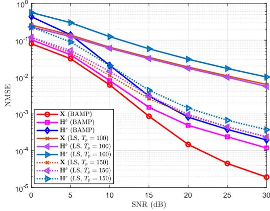
Figure 3. NMSE performance comparisons of the BAMP algorithm with baseline method (BiGAMP+LS) versus the SNR in dB for  $M = 100$ ,  $K = 500$ ,  $T = 200$  and  $N = 200$ .
