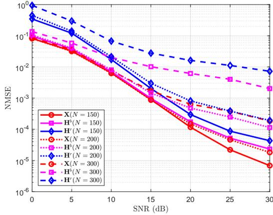
Figure 6. NMSE performance comparisons of the BAMP two-layer algorithm versus the SNR in dB for  $M = 100$ ,  $K = 500$ ,  $T = 200$  and various values of RIS elements  $N$ .
