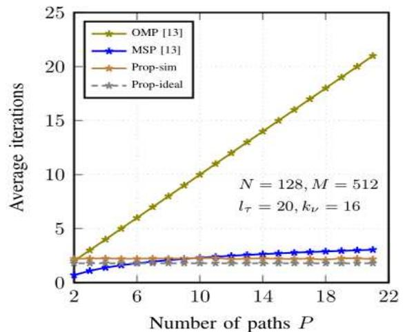
Fig. 14: Average iterations for convergence of Algorithm 1.
