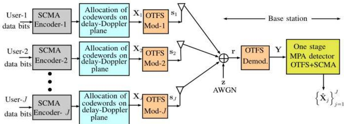
Fig. 1: Block diagram of OTFS-SCMA in uplink.
