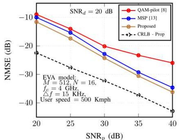
Fig. 12: NMSE of channel estimation in uplink.
