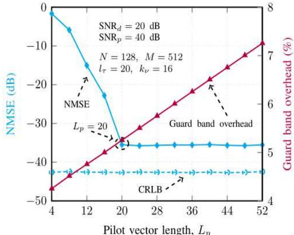
Fig. 10: Optimal pilot vector length of proposed method.
