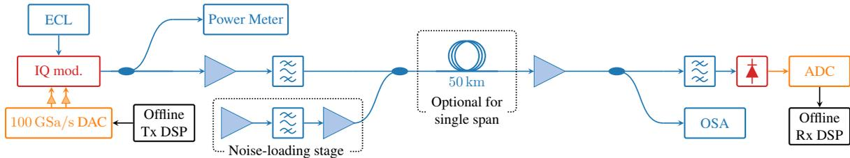
Fig. 2: Used experimental setup. A tone from an external cavity laser (ECL) is modulated by a modulator which modulates both the signal and the CW tone needed for KK detection. A single photodiode is used at the receiver.
