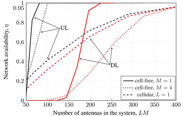
Fig. 1: Network availability for  $\epsilon_{\text{target}} = 10^{-5}$  with MMSE combining/precoding as a function of the total number of antennas in the system  $LM$ . Here,  $K = 40$ ,  $n_p = 40$ ,  $\Delta = 25^\circ$ , the scenario size is  $150 \times 150 \text{ m}$ ,  $\rho^{ul} = \rho^{dl} = -10 \text{ dBm}$ ,  $\log_2 m = 160$ , and  $n = 300$ .
