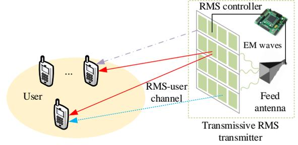
Fig. 1. MISO system based on transmissive RMS transmitter.
