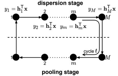
Fig. 3. Illustration of the dispersion and pooling stages. The pooling stage is depicted by mirroring the nodes. The algebraic equations of  $\mathbf{y} = \mathbf{H}\mathbf{x}$  are indexed by the nodes of the flat-tree in Fig. 1. A cycle  $t \in \{1, 2, \dots, T\}$  can be seen as the loop defined by the sequential realization of dispersion and pooling stages.
