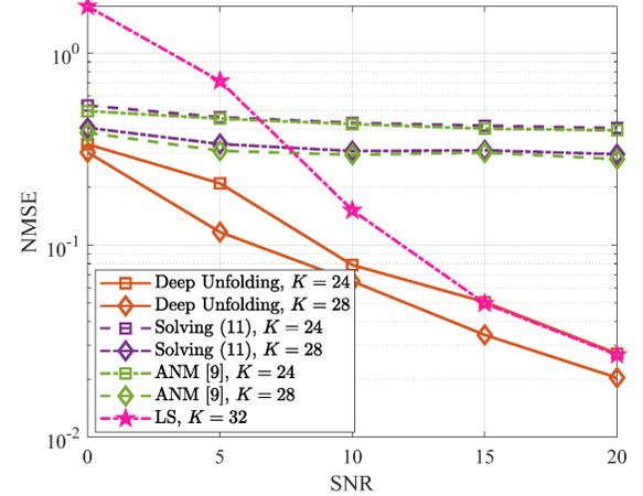
Fig. 4: Impact of training overhead on estimating the cascaded channel for a  $1 \times 16$  SIMO system with  $N = 32$  and  $L_1 = L_2 = 1$ . Deep unfolding vs. LS estimation, ANM [9], and the direct solution of (11).
