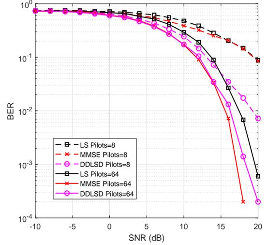
Fig. 3. BER performance under different pilot numbers.
