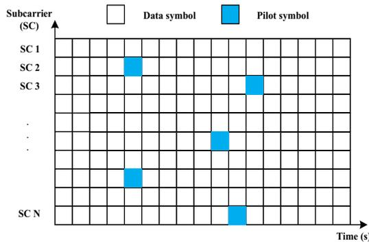
Fig. 1. The OFDM transmit symbol.
