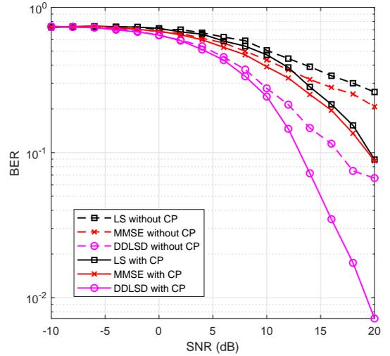
Fig. 4. Comparison of BER performance with and without CP.
