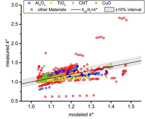
**Figure 1.** Experimentally measured versus modeled normalized thermal conductivity ( $k^*$ ) for ethylene glycol-based nanofluids. The ideal values of  $k^*$  and a  $\pm 10\%$  interval are displayed as a solid line and a grey area, respectively. Colors are used to distinguish single materials (analyzed separately) from other materials (see the legend).
