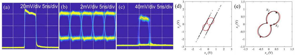
Fig. 2. (a) Optical pulses (b) Random binary signal of 200Mbps (c) Sampled Signal (d) Mixed signal and 2<sup>nd</sup> order moment (e) Comparison of theoretical 2<sup>nd</sup> order moment (black) and experimental 2<sup>nd</sup> order moment (red).
