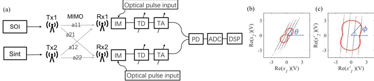
Fig. 1. (a) BSS system schematic (IM: optical intensity modulator, TD: tunable optical delay, TA: tunable optical attenuator, PD: photodetector, ADC: analog to digital conversion, DSP: digital signal processing) (b) black dots: mixed signals; red line: 2<sup>nd</sup> order moment (c) black dots: whitened signals; red line: 4<sup>th</sup> order moment.
