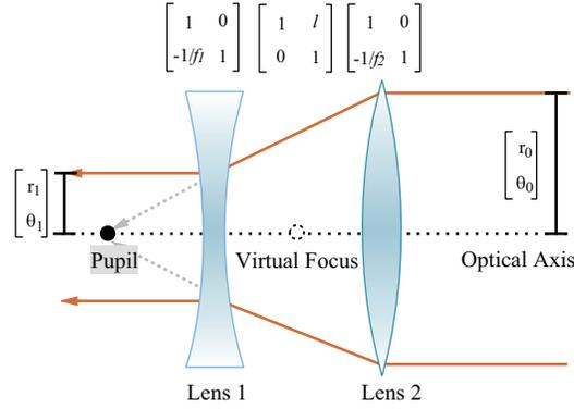
Fig. 3. Telescope internal modulator structure
