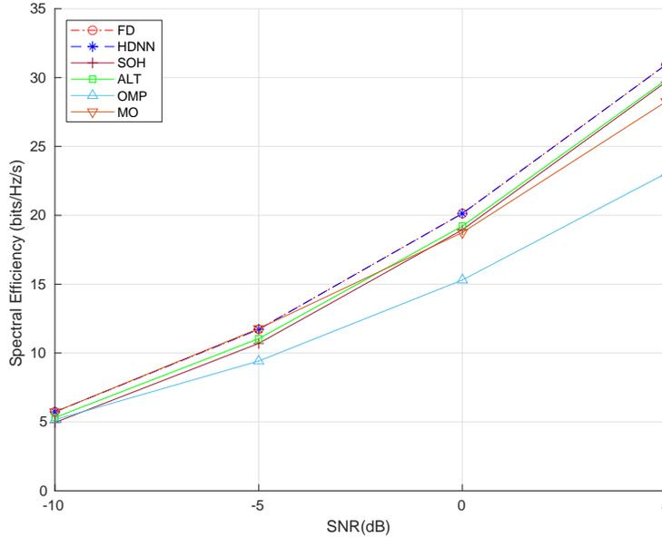
Fig. 9: Spectral efficiency versus SNR of different methods for downlink connection of  $N = 64$  massive-MIMO BS and a UE with  $M = 4$  antennas. This result has not been reported in the literature before.
