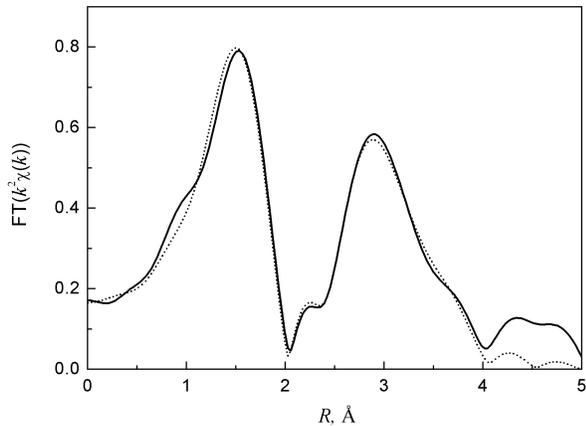
FIG. 4. Comparison of Fourier transform amplitudes for a typical EXAFS spectrum of the  $\text{Sr}_{0.98}\text{Co}_{0.02}\text{TiO}_3$  sample annealed at  $1600^\circ\text{C}$  (solid line) with the calculated curve (dotted line) corresponding to the best fit.
