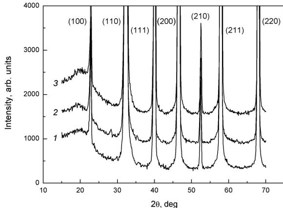
FIG. 1. X-ray diffraction patterns for the samples (1)  $\text{Sr}_{0.98}\text{Co}_{0.02}\text{TiO}_3$  annealed at  $1600^\circ\text{C}$ , (2)  $\text{Sr}_{0.98}\text{Co}_{0.02}\text{TiO}_3$  annealed at  $1500^\circ\text{C}$ , (3)  $\text{SrTi}_{0.97}\text{Co}_{0.03}\text{O}_3$  annealed at  $1500^\circ\text{C}$ .
