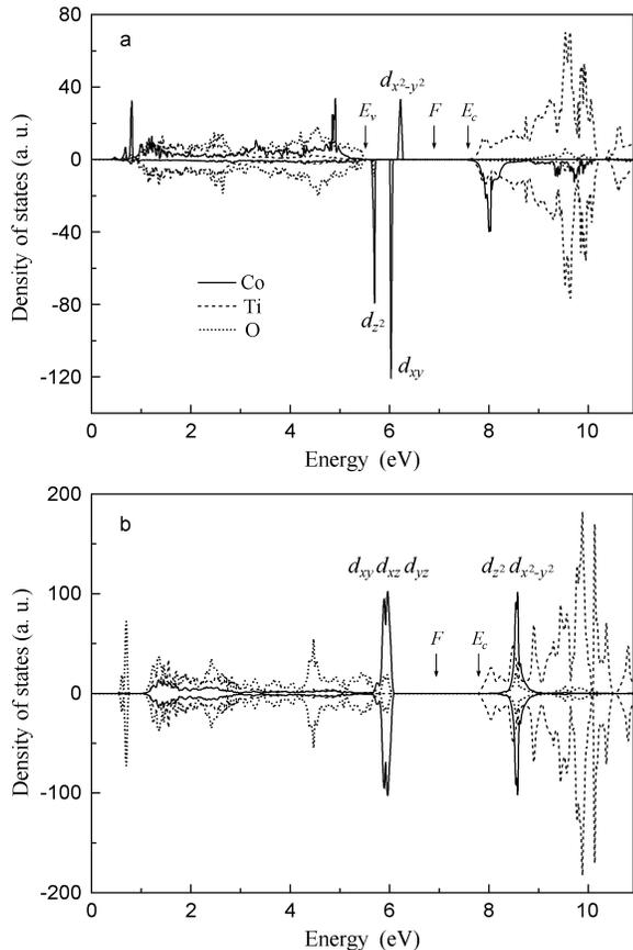
FIG. 3. Partial contributions of cobalt, titanium, and oxygen to the density of states for (a)  $\text{Co}_A^{2+}$  and (b)  $\text{Co}_B^{3+}$  impurity centers. Partial contribution of cobalt was decreased by 5 times.
