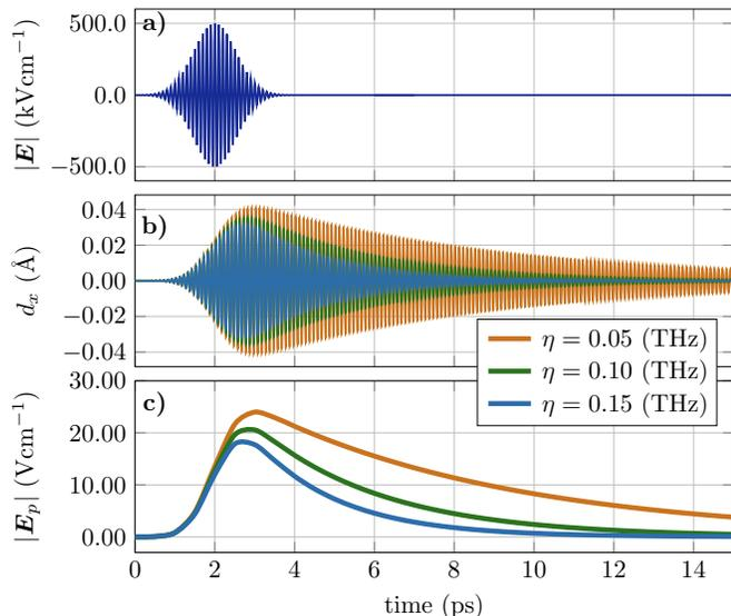
FIG. 2. (a) initial laser pulse, (b)  $x$ -component of the atomic displacement, and (c) electric field strength corresponding to the centrifugal force for a generic vibrational model. The peak of the centrifugal force arises after the peak of the initial laser pulse. Also, the lifetime of the centrifugal force is much longer than the laser pulse, depending on the material specific damping.
