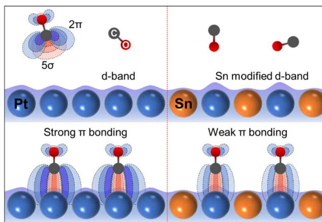
**Fig. 4.** Schematic illustration of the role of Sn on CO adsorption mechanism in Pt and Pt-Sn alloy
