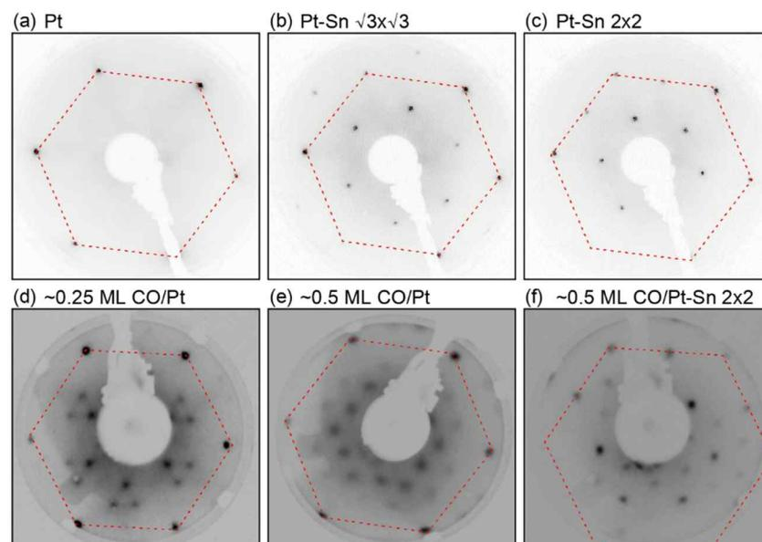
**Fig. S1.** LEED patterns of Pt(111), Pt-Sn/Pt(111)  $\sqrt{3}\times\sqrt{3}$  surface alloy, and Pt-Sn/Pt(111)  $2\times 2$  surface alloy, and changes in the surface arrangement by CO adsorption: (a) Pt(111), (b) Pt-Sn/Pt(111)  $\sqrt{3}\times\sqrt{3}$ , (c) Pt-Sn/Pt(111)  $2\times 2$ , (d)  $\sim 0.25$  ML CO/Pt, (e)  $\sim 0.5$  ML CO/Pt, and (f)  $\sim 0.5$  ML CO/Pt-Sn/Pt(111)  $2\times 2$ . Dotted lines indicate the Brillouin zone boundary.
