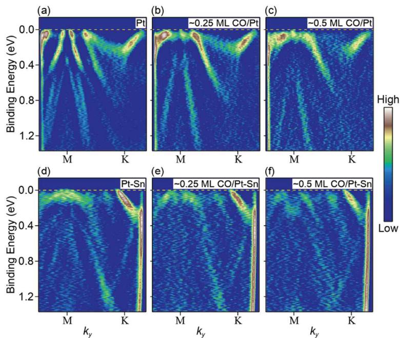
**Fig. S5.** The second derivatives of CO-induced energy band shifts are shown at the M point of (a) Pt(111), (b) ~0.25 ML CO/Pt(111), (c) ~0.5 ML CO/Pt(111), (d) Pt-Sn/Pt(111) surface alloy, (e) ~0.25 ML CO/Pt-Sn/Pt(111) surface alloy, and (f) ~0.5 ML CO/Pt-Sn/Pt(111) surface alloy.
