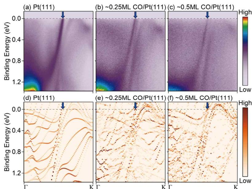
**Fig. S4.** Band structures of (a) Pt(111), (b)  $\sim 0.25$  ML CO/Pt(111), and (c)  $\sim 0.5$  ML CO/Pt(111) along the  $\Gamma$ K direction, and DFT calculation of (d) Pt(111), (e)  $\sim 0.25$  ML CO/Pt(111), and (f)  $\sim 0.5$  ML CO/Pt(111) along the  $\Gamma$ K direction. The hexagonal bands are marked with blue arrows.
