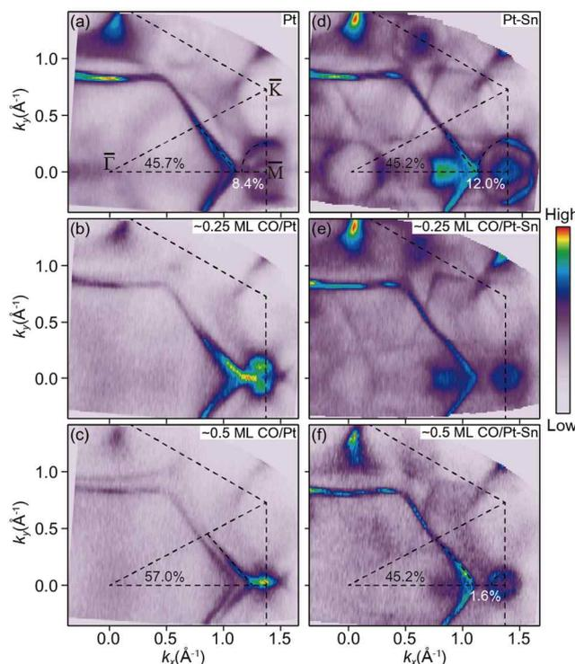
**Fig. 2.** The pristine Fermi surfaces of Pt(111) and the Pt-Sn/Pt(111)  $2 \times 2$  surface alloy are shown along with changes in the Fermi surfaces caused by CO adsorption. Fermi surface maps are shown for (a) Pt(111), (b)  $\sim 0.25$  ML CO/Pt(111), (c)  $\sim 0.5$  ML CO/Pt(111), (d) Pt-Sn/Pt(111) surface alloy, (e)  $\sim 0.25$  ML CO/Pt-Sn/Pt(111) surface alloy, and (f)  $\sim 0.5$  ML CO/Pt-Sn/Pt(111) surface alloy. Dashed lines indicate the Brillouin zone boundary.
