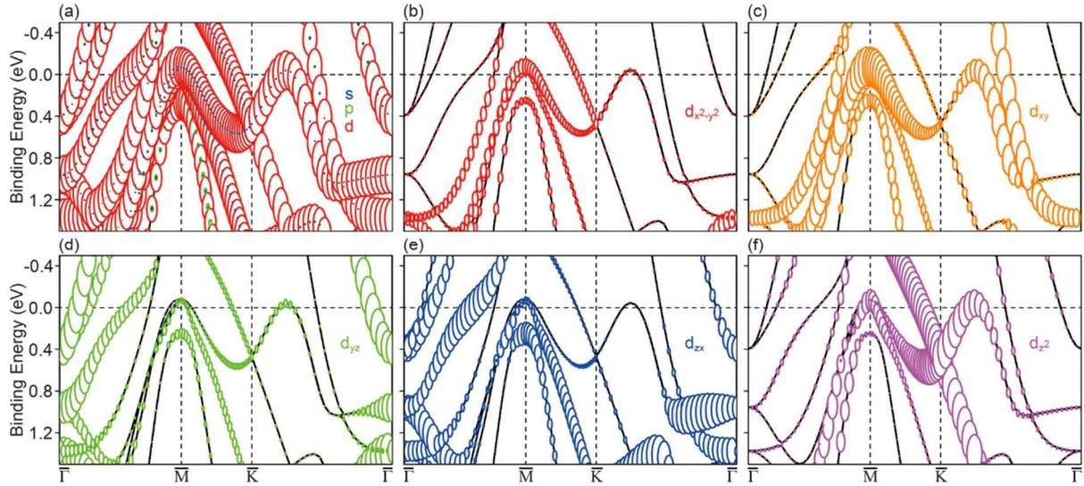
**Fig. S3.** Orbital character calculations of Pt(111). Orbital contributions of (a) s, p, d, (b)  $d_{x^2-y^2}$ , (c)  $d_{xy}$ , (d)  $d_{yz}$ , (e)  $d_{zx}$ , and (f)  $d_{z^2}$  orbitals are indicated by circles proportional to the contribution.
