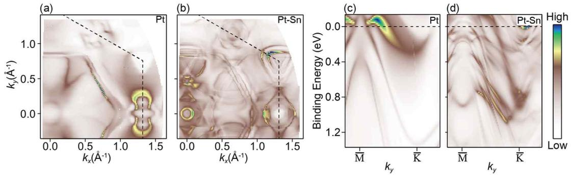
**Fig. S2.** (a) Pt, and (b) Pt-Sn/Pt(111)  $2\times 2$  surface alloy Fermi surfaces and band structures of (c) Pt, and (d) Pt-Sn/Pt(111)  $2\times 2$  surface alloy near the M point obtained with ARPES simulation.
