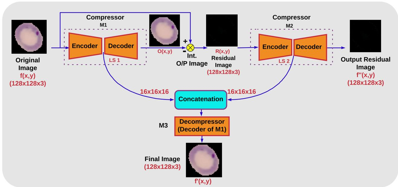
Fig. 1. Block diagram of the proposed compression-decompression model.
