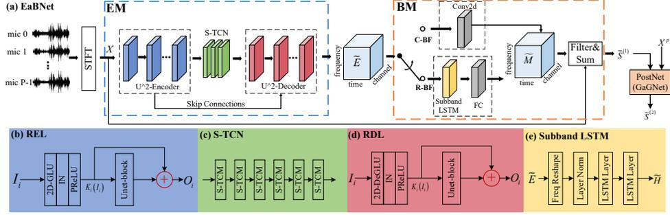
**Fig. 1.** The diagram of the proposed framework EaBNet. It mainly consists of two modules, namely EM and BM. Besides, the post-processing module is also introduced to further suppress the residual noise component. Different modules are remarked with different colors.
