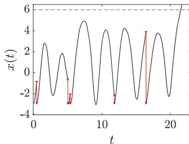
Figure 9: Time series for a realization of the process defined by  $\ddot{x} + 0.1\dot{x} + 6x - x^2 = \xi(t)$ , with resetting at exponentially distributed times. After five resetting events (red), the trajectory crosses the horizontal dotted line that marks the top of the potential and escapes.
