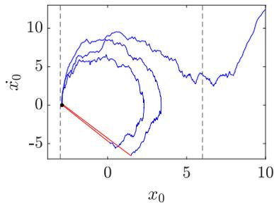
Figure 6: Trajectory in phase space for a realization of the process described by  $\ddot{x} + 0.1\dot{x} + 6x - x^2 = \xi(t)$ , with resetting at fixed time intervals of  $t_r = 2$  (red). The black point marks the initial condition  $x_0 = -2.899$  and the vertical dotted lines denote the ends of the potential ( $x^-$  and  $x_+$ ). After two resetting events the particle leaves the well.
