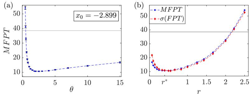
Figure 11: Mean first passage time dependence on the resetting rate. (a) The MFPT is represented against  $\theta = 1/r$ . The minimum corresponds to a mean resetting interval slightly above the deterministic resetting  $t_r^*$  value. (b) The MFPT and the standard deviation are equal for the optimal rate,  $r = r^* = 0.4$ .
