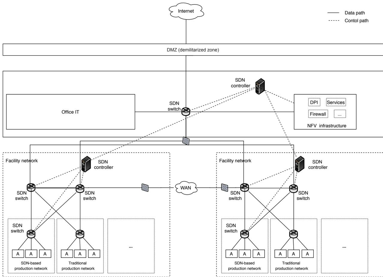
Fig. 3. Reference architecture for future IIoT networks
