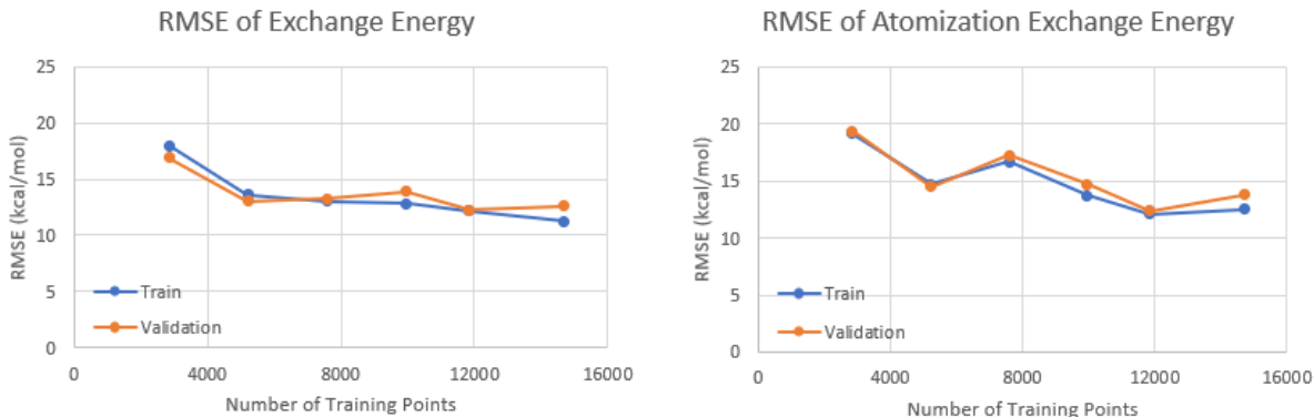
Figure S1: RMSE of Exchange Energy and Atomization Exchange Energy with respect to training set size on the Jensen validation set, for the feature set in eqs 17 and 19 and a squared-exponential (non-additive) kernel.
