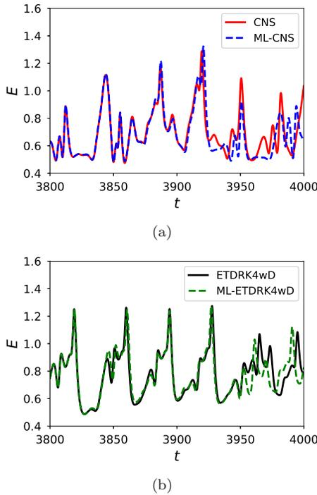
FIG. 5. Comparisons of the energy  $E(t) = \frac{1}{2L} \int_0^L U^2(x, t) dx$ . (a) Comparison between the actual result given by the CNS and the ML prediction based on the “clean database”. (b) Comparison between the actual result given by the traditional algorithm ETDRK4wD and the ML prediction based on the “polluted database”. Solid and dashed line denote the actual result and the ML prediction, respectively.
