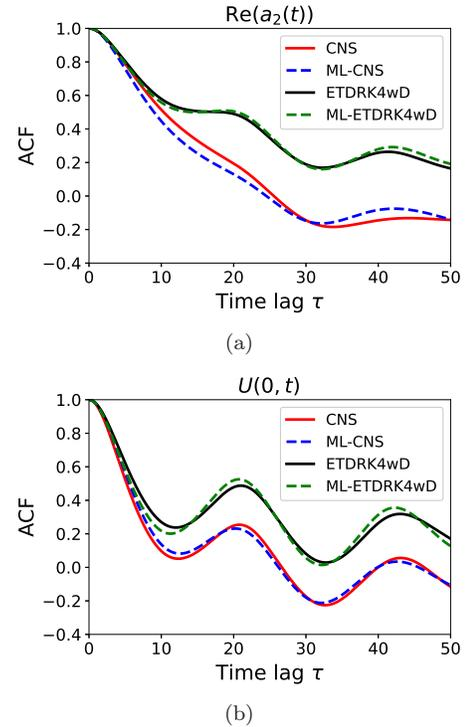
FIG. 6. Comparison of Autocorrelation functions (ACFs). (a) ACFs of  $\text{Re}(a_2(t))$ . (b) ACFs of  $U(0, t)$ . Solid line in red is the actual result given by the CNS, the solid line in black is the actual result given by the traditional algorithm ETDRK4wD, the dashed line in blue is the ML prediction based on the “clean database”, the dashed line in green is the ML prediction based on the “polluted database”, respectively.
