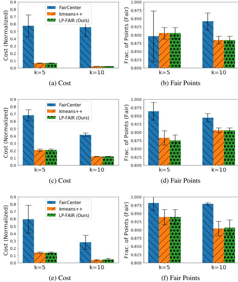
Figure 3:  **$k$ -means**: The results produced by all methods on (a-b) Bank, (c-d) Census, and (e-f) Diabetes datasets both in terms of Cost (lower is better) and fraction of points that are individually fair (higher is better).
