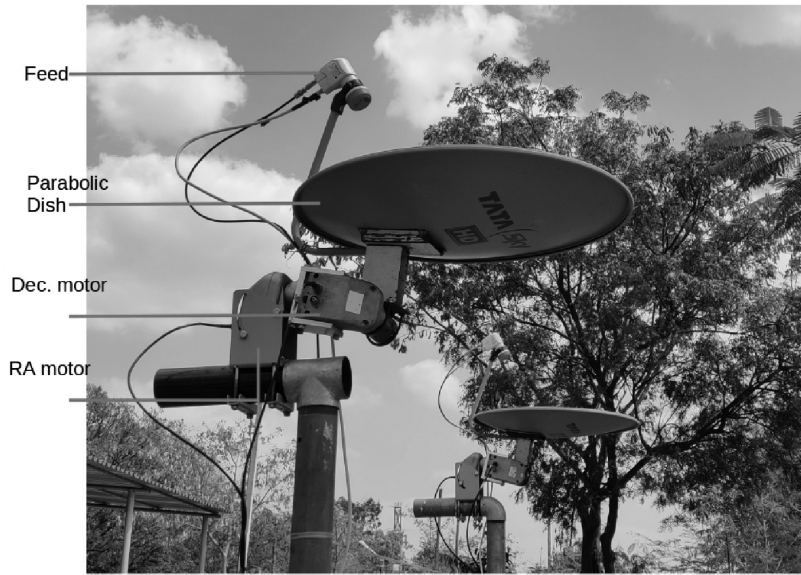
Figure 1. The commercial dish TV antennas used in the Gauribidanur observatory for solar observations in the correlation interferometer mode.
