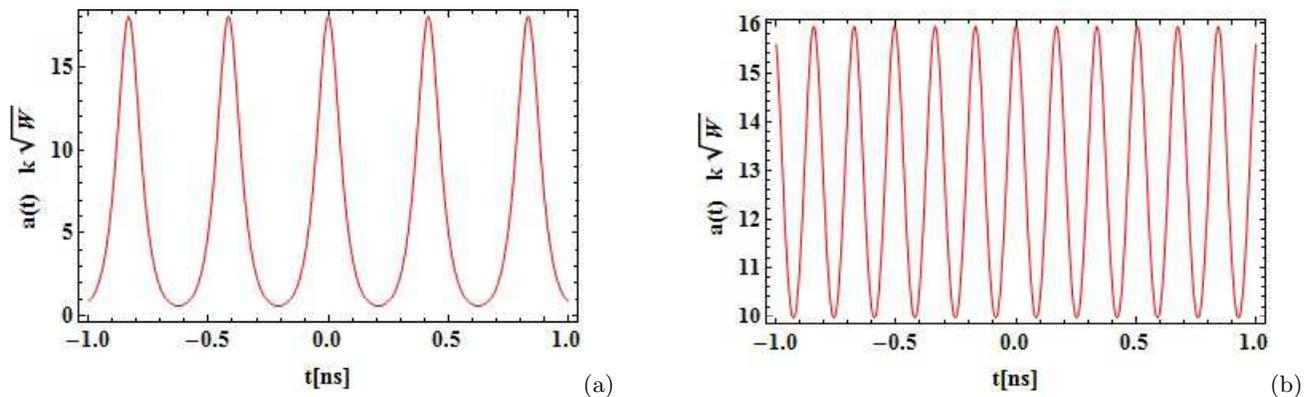
FIG. 1. Elliptic-soliton solution to the nonlinear amplitude equation (2), for two different values of the parameter of pulse dispersion  $k$ : (a) Periodic network of sharp pulse signals for large dispersion parameter ( $k = 0.98$ ), (b) Elliptic-wave decay into a quasi-continuous signal for small dispersion parameter ( $k = 0.6$ ).
