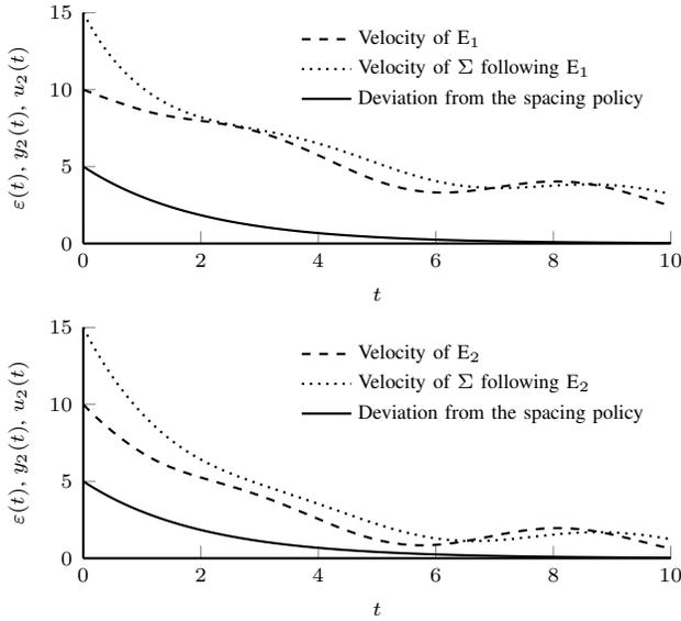
Fig. 5. For each  $i \in \{1, 2\}$ , the velocity  $u_2$  of the leading vehicle  $E_i$ , the velocity  $y_2$  of the controlled vehicle  $\Sigma$  following  $E_i$ , and the deviation from the headway spacing policy  $\varepsilon = y_1 - u_1 + h y_2$ , with  $h$  in (16) given by  $l(t) = 1$  if  $t \in [0, 1]$  and  $l(t) = \frac{1}{2} + \sin(\frac{3\pi}{8}t + \frac{3\pi}{16})$  if  $t > 1$ .
