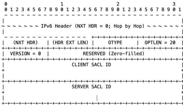
Figure 5: Packet format for transmitting SACL ID
