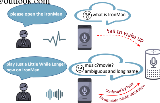
Figure 1: Iron Man can be a name of a smart device or a movie and the system would be unable to react properly upon “Please play Iron Man” from a user. Another case as “Play just a little while longer now on Iron Man” requires the system to classify “Play” between music and movie domains, and whether “now” should be combined with “just a little while longer” as a whole.
