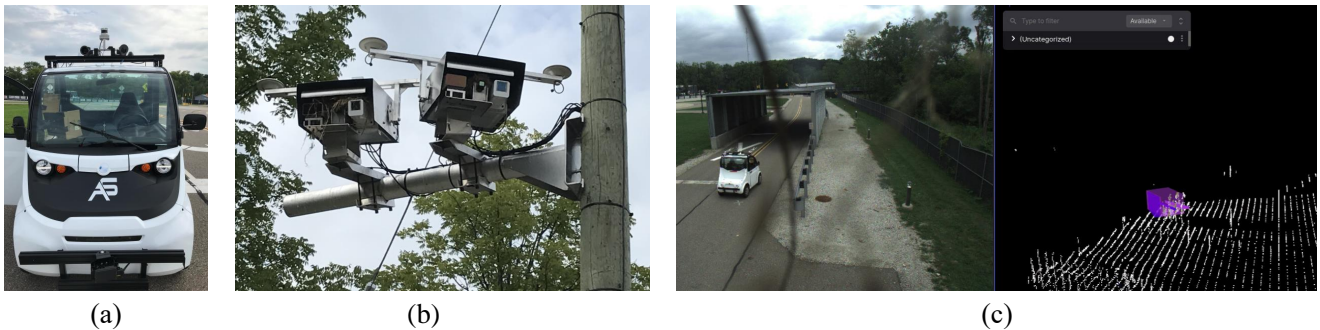
Fig. 2. Setup for ix-node perception. (a) Ford's autonomous vehicle. (b) Ix-node with sensor heads. (c) Ix-node's camera image (left) and vehicle candidate generation result as colored marker with LiDAR's point cloud (right).
