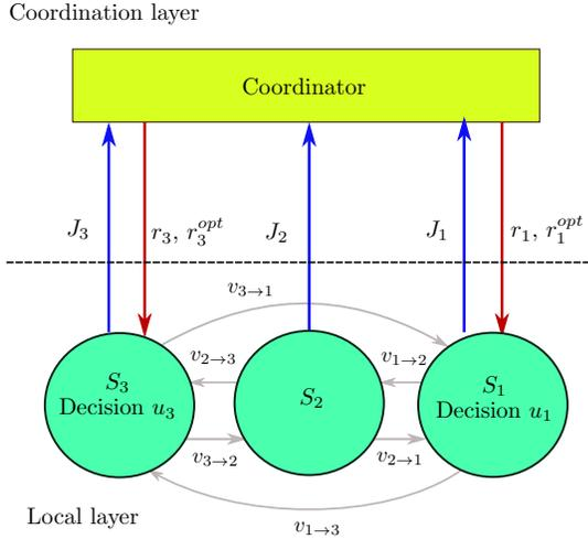
Fig. 1. Example of the hierarchical control architecture and the interconnection network between the subsystems. The presented sets correspond to this example are  $\mathcal{N} := \{1, 2, 3\}$ ;  $\mathcal{N}^{ctr} := \{1, 3\}$ ,  $\mathcal{N}_1 = \{2, 3\}$ ,  $\mathcal{N}_2 = \{1, 3\}$ ,  $\mathcal{N}_3 = \{1, 2\}$ .
