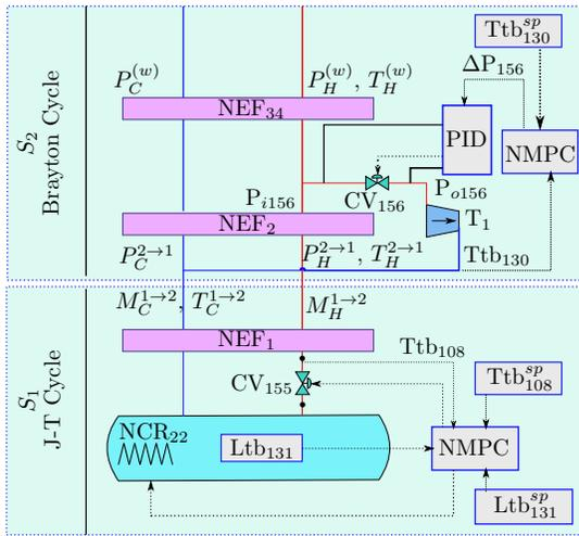
Fig. 3. Block diagram of the cold box plant.
