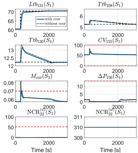
Fig. 7. Comparison of the system behavior between using the hierarchical control and observer-based decentralized control. In this scenario, the set-point of liquid helium level  $Ltb_{131}$  is changed at instant  $t = 300$ . Under decentralized control, although  $Ltb_{131}$  tracks the set-point faster than the one given by hierarchical control, the constraint on  $M_{out}$  is violated, which is not the case with the coordination.
