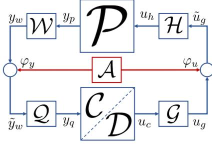
Fig. 1: Block diagram of the closed-loop cyber-physical system, including plant  $\mathcal{P}$ , controller  $\mathcal{C}$  and watermarking filters  $\{\mathcal{W}, \mathcal{Q}\}$  and  $\{\mathcal{G}, \mathcal{H}\}$ . Signals transmitted between the plant and the controller may be altered by an attacker  $\mathcal{A}$ .
