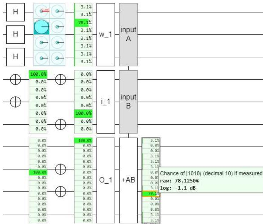
Fig. 4.b. Quantum neural network – result received by changing the input neuron value after training the neural network.
