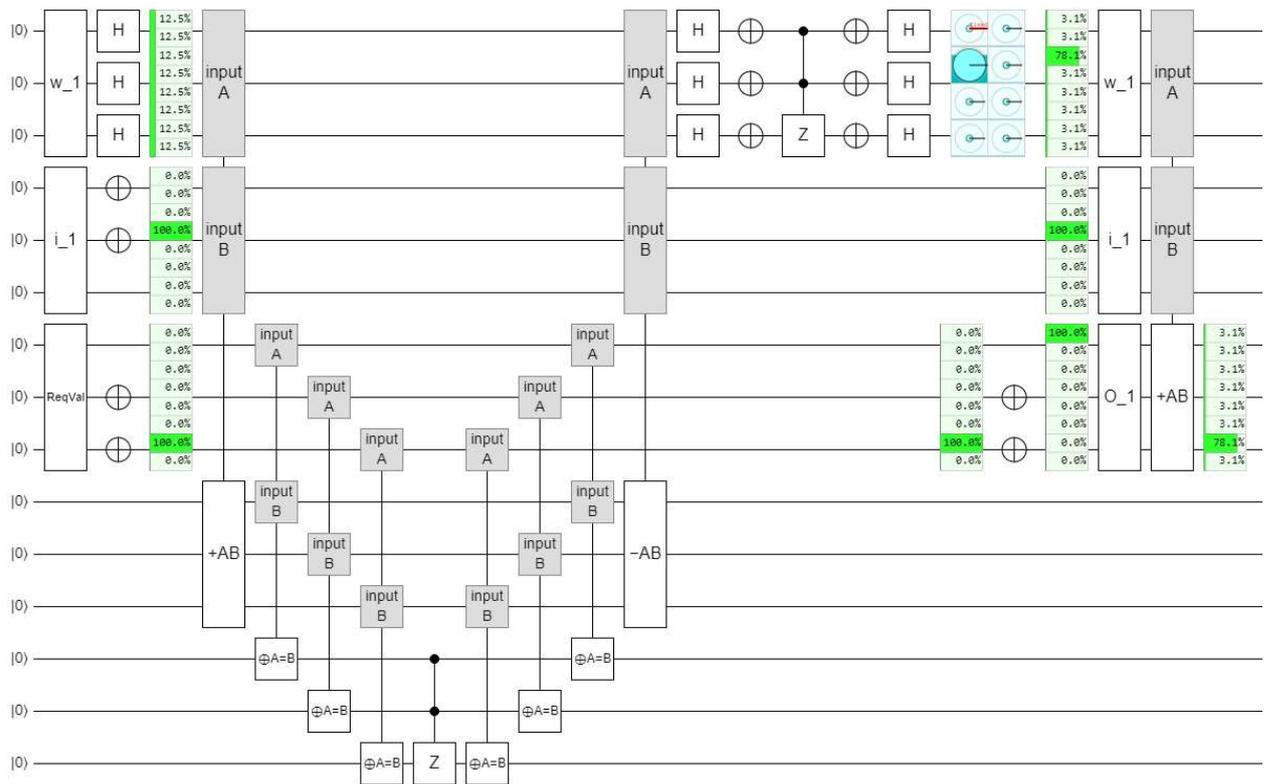
Fig. 3.a. Quantum neural network – running the training algorithm and verifying the results<sup>1</sup>
