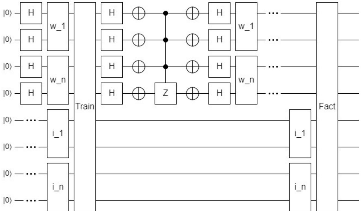
*Fig. 5. The proposed concept of constructing quantum neural networks based on Grover's algorithm.*
