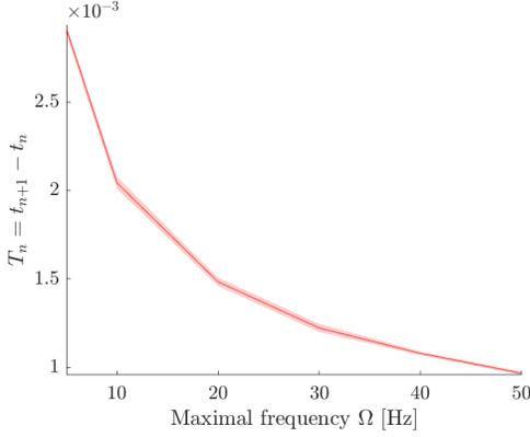
**Fig. 3.** Time instances differences in IF-TEM with BL signals as a function of the frequency band. The solid line shows the average  $T_n$  and the shaded region captures the standard deviation. See the range in Table 1.
