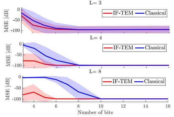
**Fig. 4.** Mean-squared error in estimating an FRI signal as a function of the number of bits. The solid line shows the average error and the shaded region captures the standard deviation in the estimate.
