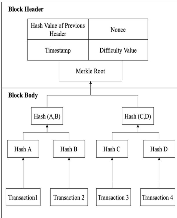
Fig. 2. Structure of block.
