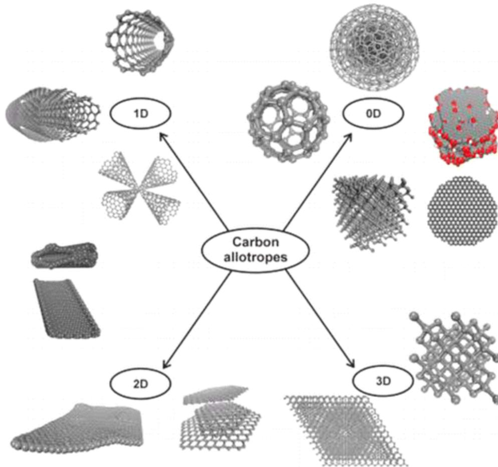
**Fig. 1** Structures of different forms of carbon allotropes (**Reproduced with permission from [21]**)
