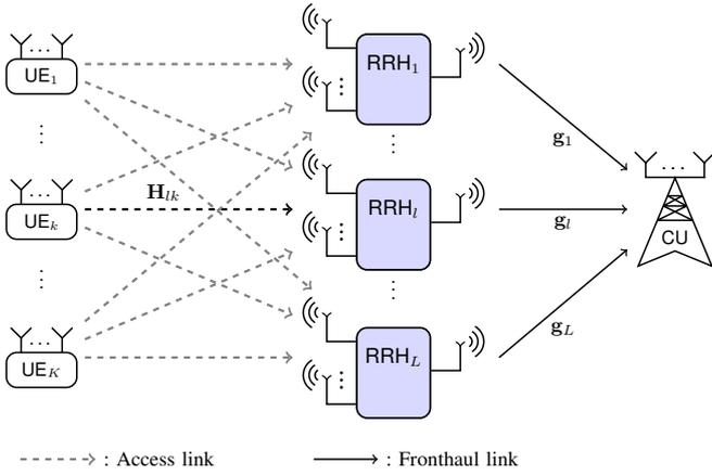
Fig. 1. The schematic diagram of the C-RAN system utilizing massive MIMO fronthaul.
