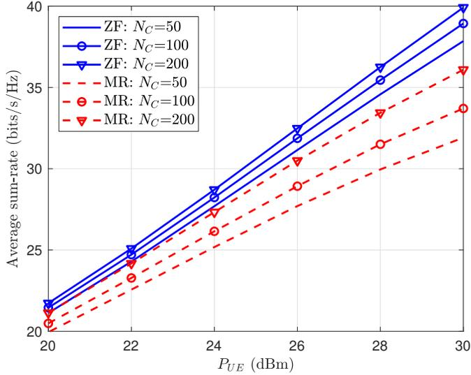
Fig. 3. The average sum-rate with respect to the UE transmit power  $P_{UE}$  for for MR and ZF combining schemes, and for different number of antennas at the CU  $N_C$  with  $K = 10$ ,  $L = 4$ ,  $N_{U,k} = 2$ ,  $N_{H,l} = 3$ , and  $P_H^{\max} = 30$  dBm.
