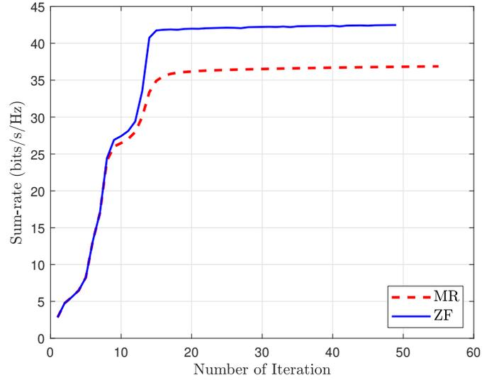
Fig. 2. The convergence of the proposed algorithm for MR and ZF fronthaul beamforming with  $K = 4, L = 4, N_{U,k} = 2, N_{H,l} = 2$  and  $N_C = 200$ .
