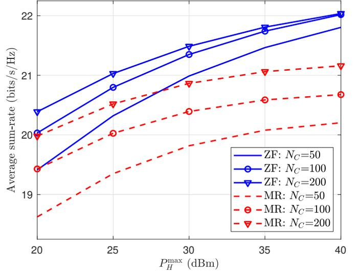
Fig. 4. The average sum-rate with respect to the maximum available transmit power at RRHs  $P_H^{\max}$  for for MR and ZF schemes, and for different number of antennas at the CU  $N_C$  with  $K = 10$ ,  $L = 4$ ,  $N_{U,k} = 2$ ,  $N_{H,l} = 3$ , and  $P_{UE} = 20$  dBm.
