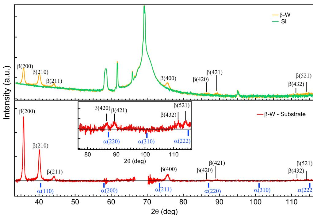
Fig. S5.  $\theta - 2\theta$  x-ray diffraction pattern of (a) tungsten thin film grown on Si(001)+SiO<sub>2</sub> substrate and the Si substrate. (b) W XRD after subtracting the substrate intensity measured under exactly the same condition as the thin film. The  $\beta$ -W peaks are marked in black and position of  $\alpha$ -W peaks as shown with blue marker. The inset show zoomed-in view of diffraction intensity from 76° - 116°
