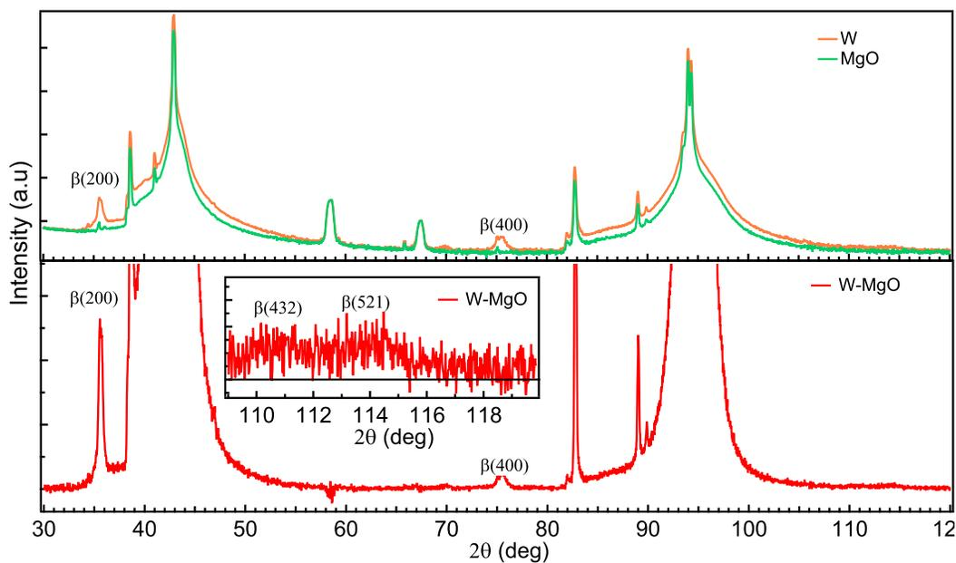
Fig. S6.  $\theta - 2\theta$  x-ray diffraction pattern of (a) tungsten thin film grown on MgO substrate and the MgO. (b) W XRD after subtracting the MgO intensity measured under exactly the same condition as the thin film. The  $\beta$ -W peaks are marked in black and position of  $\alpha$ -W peaks as shown with blue marker. The inset show zoomed-in view of diffraction intensity from 109° - 120°
