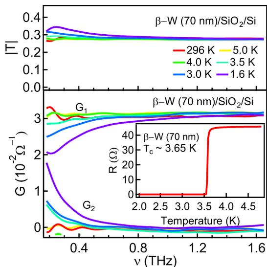
FIG. 1. (Top) Zero-field magnitude of transmission, (Bottom) Real  $G_1(\nu)$  and imaginary  $G_2(\nu)$  parts of the zero-field complex conductance of  $\beta$ -W 70 nm thin film grown on Si substrate as a function of frequency from room temperature ( $T \gg T_c$ ) to (1.6 K  $\ll T_c$ ). Inset: Temperature dependence of the 4-probe dc resistance.
