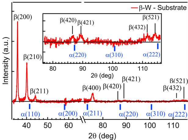
FIG. 6.  $\theta - 2\theta$  x-ray diffraction pattern of tungsten thin film grown on Si(001)+SiO<sub>2</sub> substrate after subtracting the substrate intensity measured under exactly the same condition as the thin film. The  $\beta$ -W peaks are marked in black and position of  $\alpha$ -W peaks as shown with blue marker. The inset show zoomed-in view of diffraction intensity from 76° - 116°.
