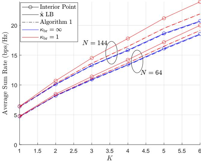
Fig. 3: Average sum-rate using numerical optimization, the AO algorithm and the lower bound for varying numbers of UEs,  $N \in \{64, 144\}$ ,  $\kappa_d = \kappa_{ru} = 1$ ,  $\kappa_{br} \in \{\infty, 1\}$ .
