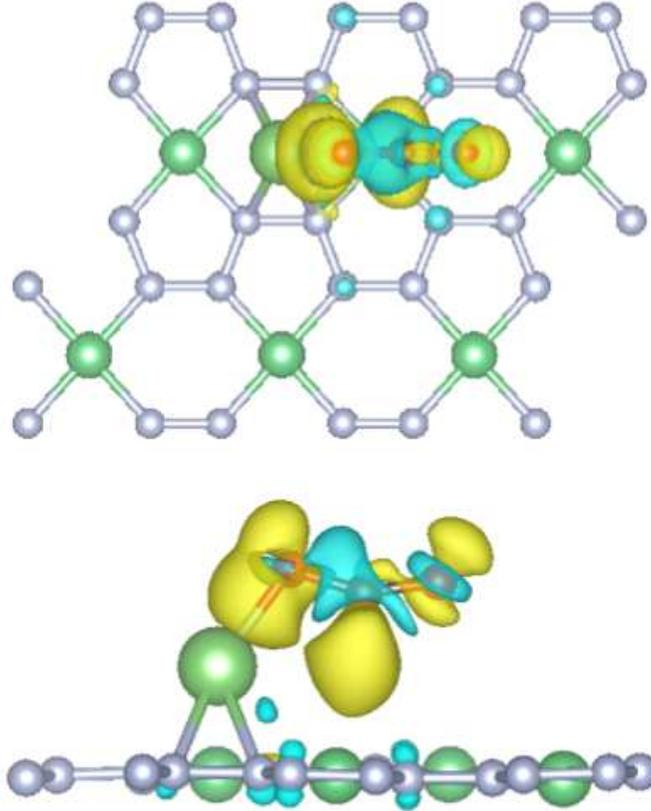
FIG. 7: Top and side view of charge transfer isosurface for adsorption of CO<sub>2</sub> on Li-doped beryllonitrene. Yellow areas are charge gained and blue areas are charge lost.
