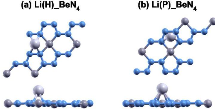
FIG. 4: Optimized atomic structure of beryllonitrene  $2 \times 2$  supercell doped with Li at (a) H (above the center of the  $\text{Be}_2\text{N}_4$  hexagon) and at (b) P (above the center of the  $\text{BeN}_4$  pentagon) after relaxation. The blue atoms are nitrogen, the dark grey atoms are beryllium, and the light grey atoms are lithium.
