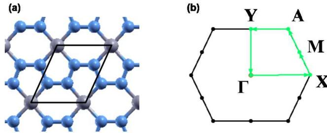
FIG. 1: (a) Atomic structure of pristine beryllonitrene. The black frame indicates a  $1 \times 1$  cell (b) First Brillouin zone for beryllonitrene with high symmetry points  $\Gamma$ , X, M, A, and Y<sup>55</sup>.
