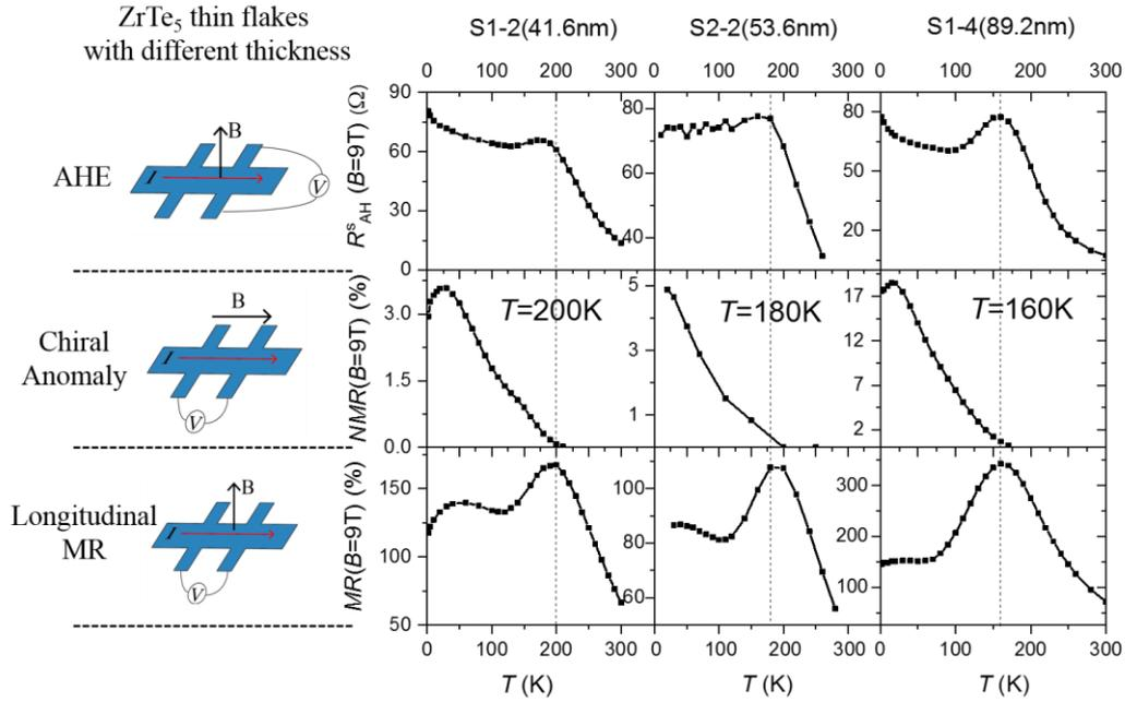
Figure 4. Summary of temperature dependent  $MR$  at different measurement configurations. The upper panel shows the saturated Hall anomaly  $R_{AH}^s(B = 9T)$  with out-of-plane magnetic field. The middle panel represents the amplitude of negative magneto-resistance  $NMR(B = 9T)$  with magnetic field parallel to the direction of current. The lower panel depicts the longitudinal magneto-resistance  $MR(B = 9T)$  with out-of-plane magnetic field.
