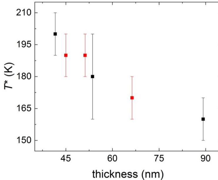
Figure 5. The dependence of  $T^*$  on  $ZrTe_5$  sample thickness.  $T^*$  decreases monotonically from 200K to 160K with increasing thickness of the  $ZrTe_5$  thin flakes from 42nm to 89nm. Here black squares are measured from crystals purchased from PrMat Technology company [www.prmat.com] and red squares are measured from crystals obtained from Brookhaven National Lab [19].
