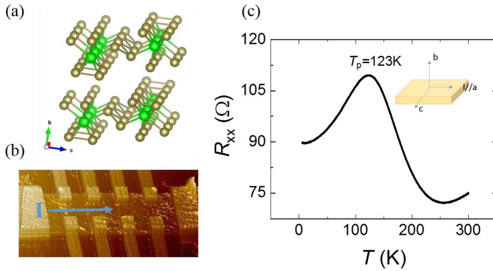
Figure 1. Illustration and characterization of device. (a) Atomic structural schematics of ZrTe<sub>5</sub>. Here green and grey balls denote zirconium and tellurium atoms, respectively. (b) 3D AFM image of a ZrTe<sub>5</sub> device with thickness of 42 nm. The blue arrow indicates the direction of electrical current. (c)  $R$ - $T$  curve of the device at zero magnetic field. Inset: crystal orientation and current of the ZrTe<sub>5</sub> device.
