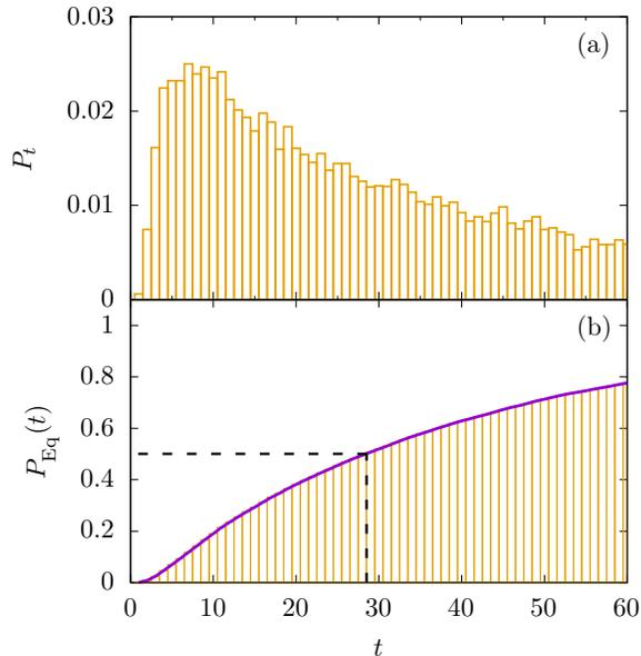
**FIG. 4:** Panel a: Occurrence probability  $P_t$  for a 16-spin chain and "SYH" process. Panel b: Cumulative probability distribution calculated by the approximation of the integral (orange boxes). Alternatively, calculated by means of  $\text{tr}[\hat{P}_{\text{Eq}} \varrho(t)]$  (solid violet line). The dashed straight line indicates the value of  $t_{1/2}$  obtained when  $\hat{P}_{\text{Eq}} = 1/2$ .
