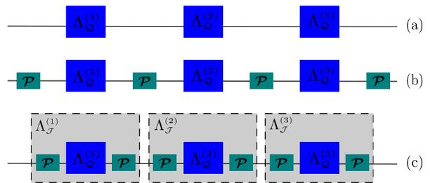
**FIG. 1:** Conversion of the three-time step quantum process  $\Lambda_{\mathcal{Q}}$  consisting of the CPTP maps  $\Lambda_{\mathcal{Q}}(n)$  shown in line (a) into a classical process by complete measurements, denoted by  $\mathcal{P}$ . The result is depicted in line (b). In line (c) the intermediate measurements are duplicated, which results in the classical maps  $\Lambda_{\mathcal{J}}(n) = \mathcal{P} \circ \Lambda_{\mathcal{Q}}(n) \circ \mathcal{P}$ .
