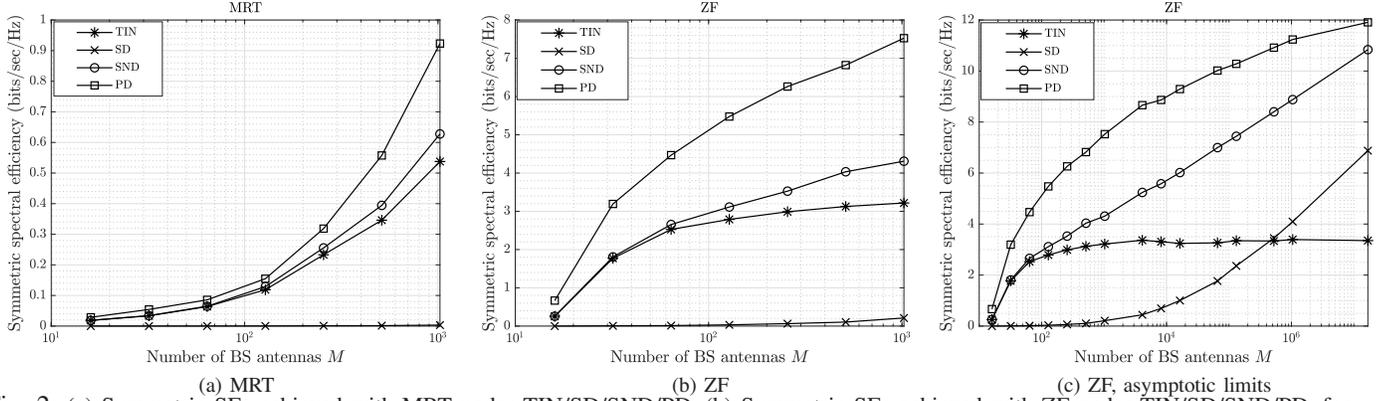
Fig. 2: (a) Symmetric SEs achieved with MRT under TIN/SD/SND/PD, (b) Symmetric SEs achieved with ZF under TIN/SD/SND/PD, for a range of moderately large  $M$ , (c) Asymptotic limits of symmetric SEs with ZF under TIN/SD/SND/PD for truly large values of  $M$ .
