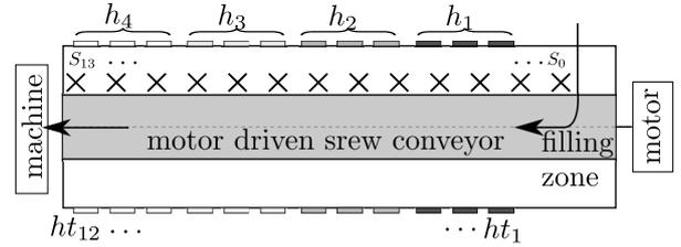
Fig. 1. A typical extruder configuration.
