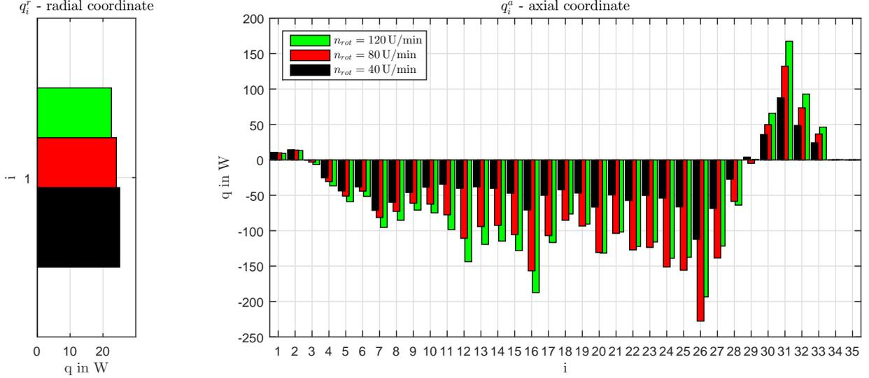
Fig. 6. Heat flow observation from experiments by the Smart Sensor, from *Granulate A* in different operating points.
