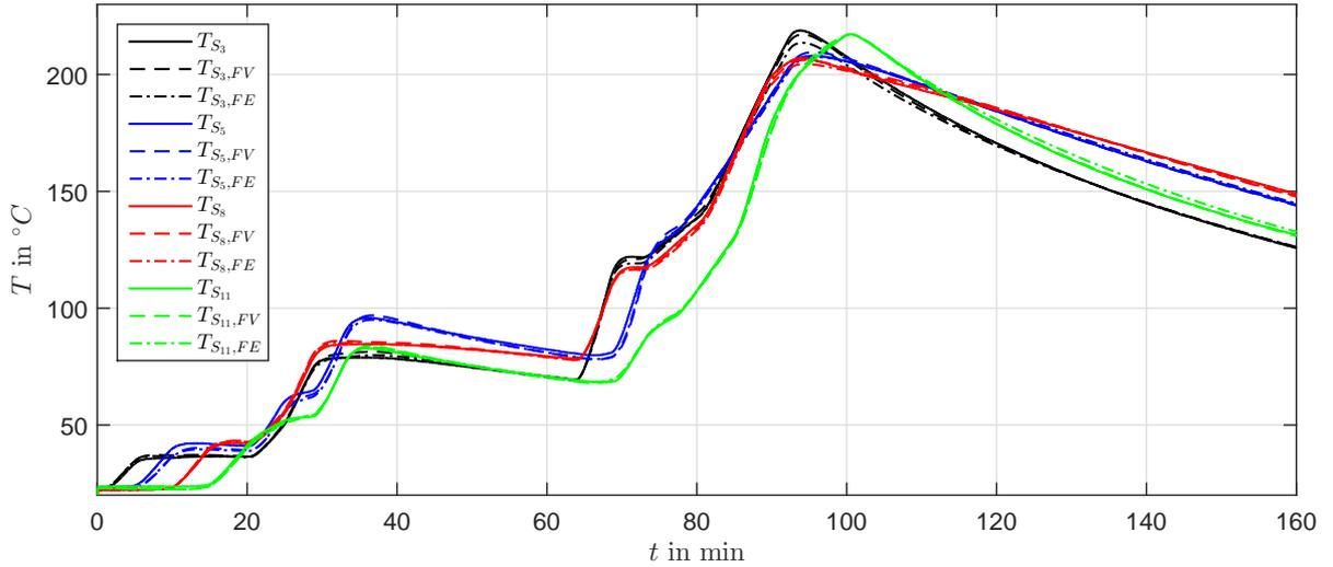
Fig. 4. Comparison between the measurement and the FV- and FE - model simulation results.
