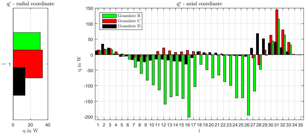
Fig. 8. Heat flow observation from extrusion experiments by the Smart Sensor, from different granulate types.
