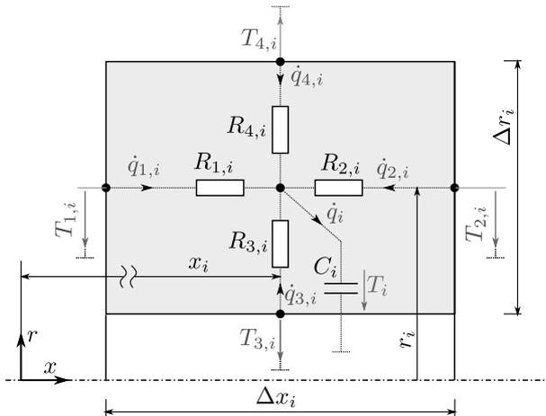
Fig. 2. Equivalent circuit for a typical extruder configuration.
