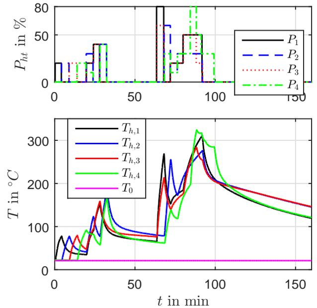
Fig. 5. Connection between percentage power  $P$  and the heating tape temperature  $T_h$ .
