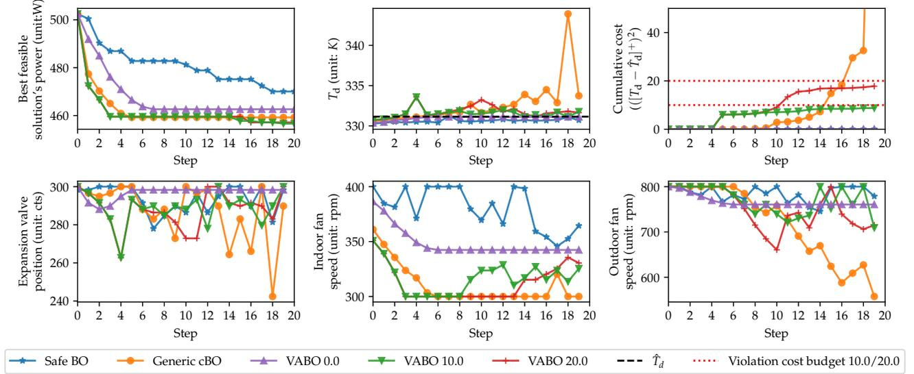
Figure 2: Best feasible solution’s power, discharge temperature, cumulative violation cost and the three set-points’ evolution.
