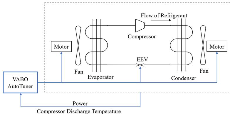
Figure 1: Schematic diagram of vapor compression system with our proposed VABO controlling the EEV (electronic expansion valve) and the two fans’ speed. For simplicity, we do not show other measurements and controls.
