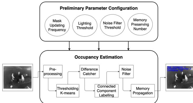
**Fig. 2.** Process flow diagram of the occupancy estimation model
