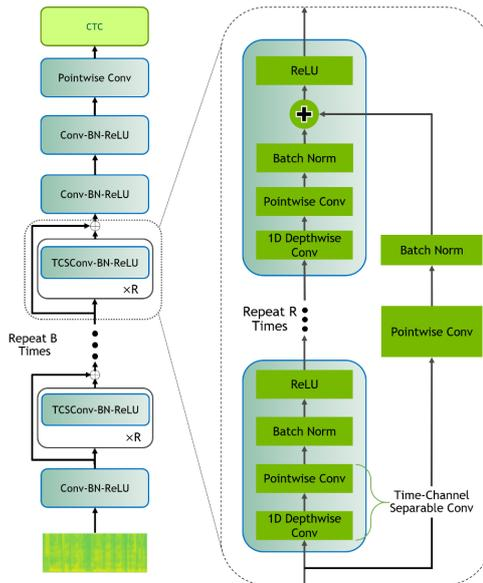
Figure 1: Network architecture of Nvidia’s QuartzNet [17].
